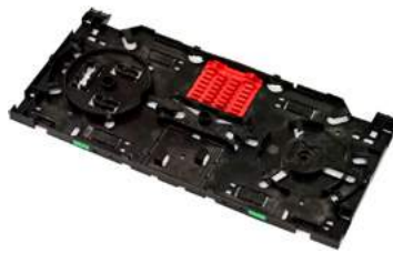
Cassette with an option for 12 fusion splices
