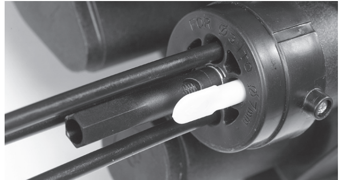
3.3.1.8 Tighten the trigger until it butts up with the flange. The spring should be hidden after tightening.
