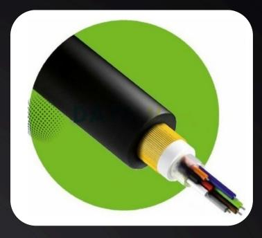
DATAWAY self-supporting 1-fibre cable with LSOH sheath (UV resistant) and fibre type G.657A1 is designed for outdoor and indoor use in FTTx systems. The cable is reinforced with aramid fibers, lightweight construction with a small diameter of 3.1 mm.
